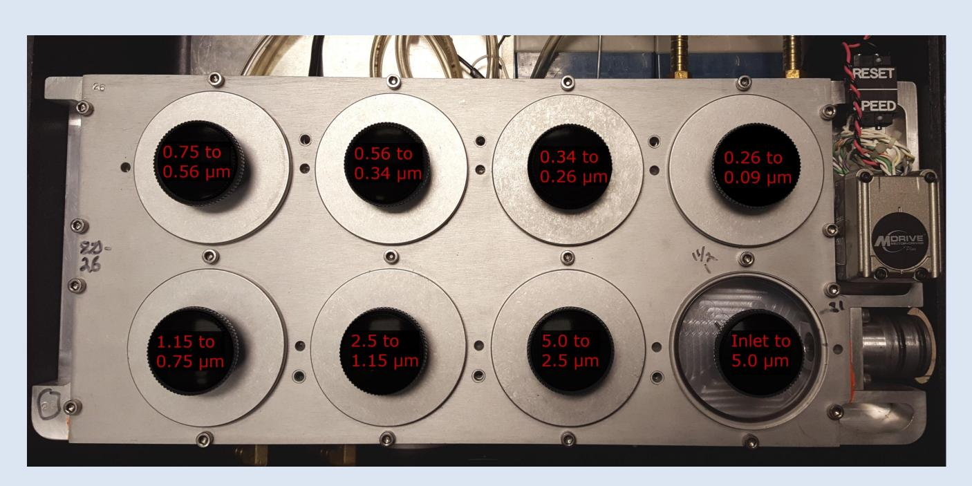
Size- and Time-Resolved Sampling Coupled with Nuclear Analysis Rotating Lundgren-style impactor, 8 size cuts, 10 liters/minute with userspecified time bins. Due to very small sample loading, conventional methods for analysis cannot be used. The following methods have been developed specifically for this sampling technique.
